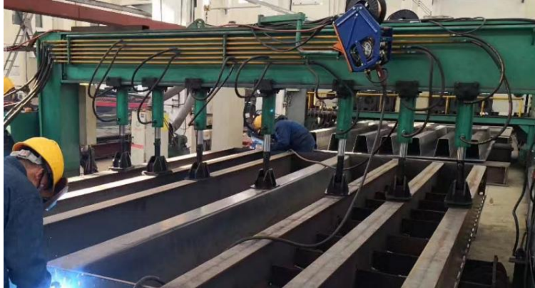
Standard fillet weld with no end, the minimum weld leg length is 8mm
