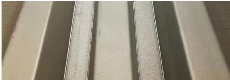
Standard fillet weld with no end, the minimum weld leg length is 8mm
